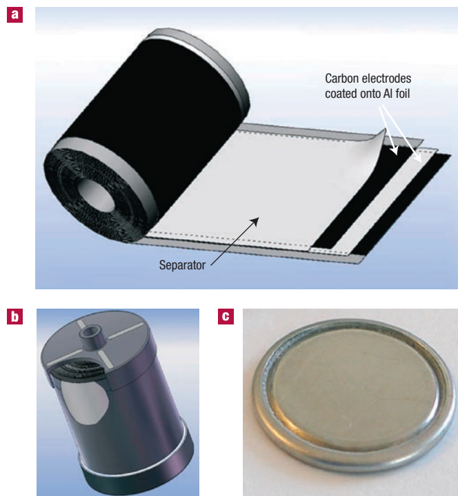
Figure 3 Electrochemical capacitors. a , Schematic of a commercial spirally wound double layer capacitor. b , Assembled device weighing 500 g and rated for 2,600 F. (Photo courtesy of Batscap, Groupe Bolloré, France.) c , A small button cell, which is just 1.6 mm in height and stores 5 F. (Photo courtesy of Y-Carbon, US.) Both devices operate at 2.7 V.
